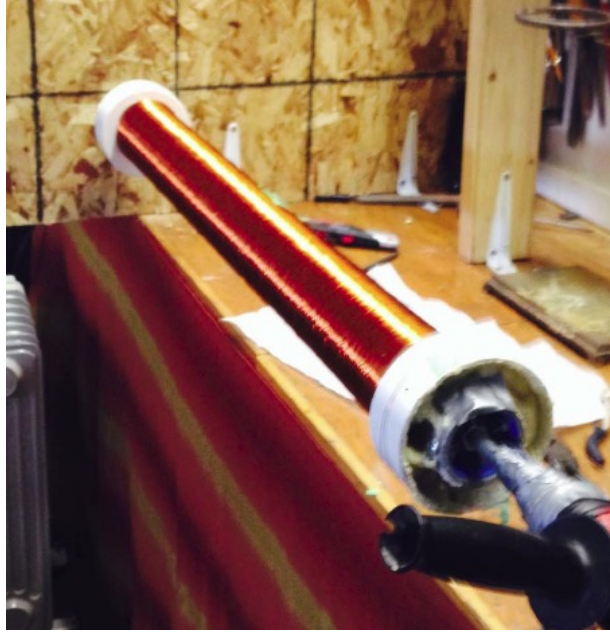
Figure 6.3 The magnetometer during stages of wrapping the copper wire. There were between 96,000 to 97,000 turns.
