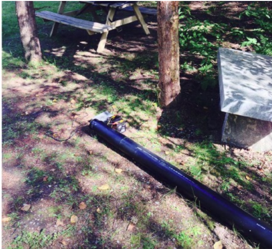
Figure 6.2 Cylinder containing the induction magnetometer “Herbert” by which local Schumann resonances were measured.
