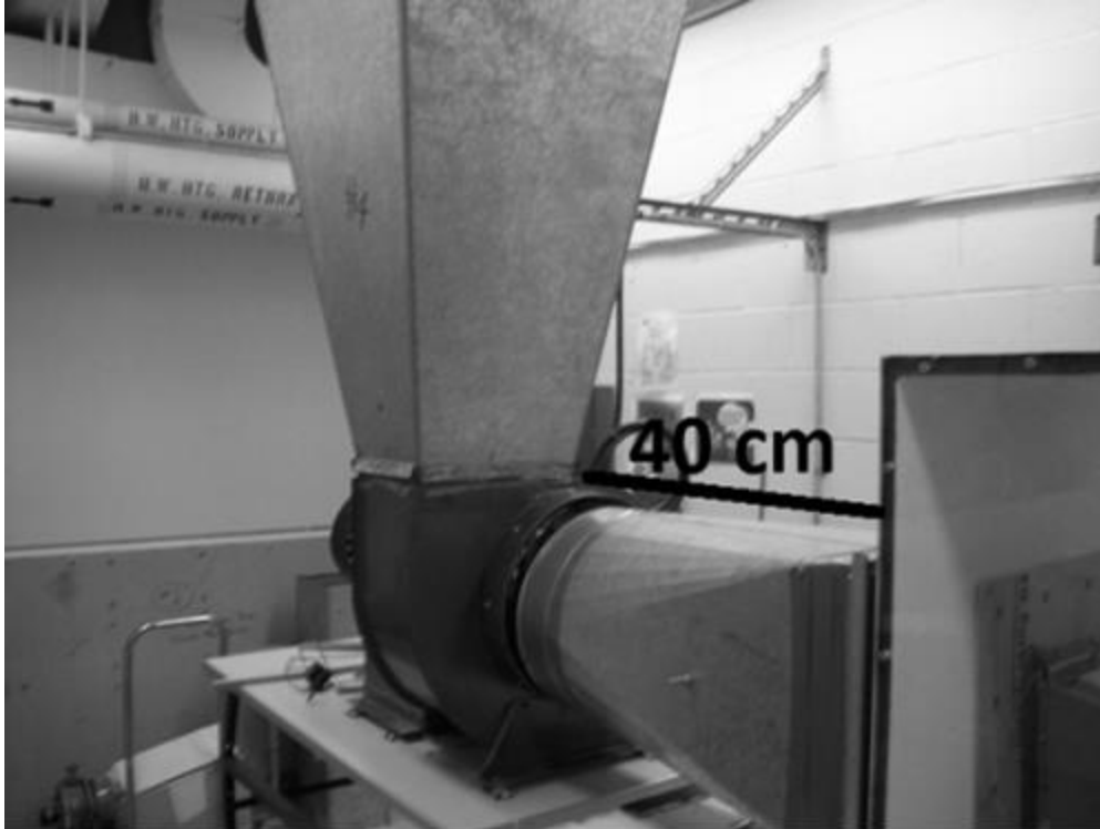
Figure 73: Post divergent duct to fan and evasee
