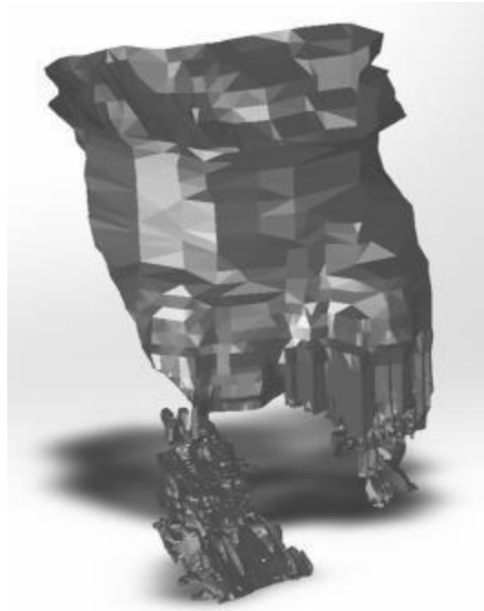
Figure 128: .stl file that was converted into a CAD/CAM solid object shell capable of being assigned porous material properties in the flow simulation tool when filled. To note, the excess image that needed to be removed from the bottom LHS is the ore deposit rising from depth.
