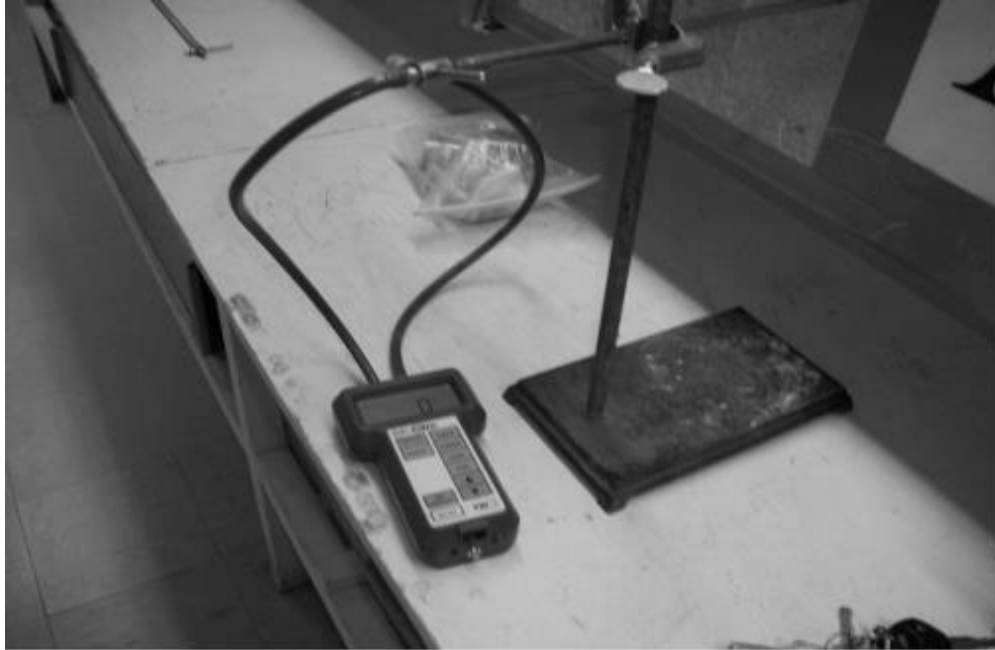
Figure 77: TSI 8705 Micromanometer used in experimentation
