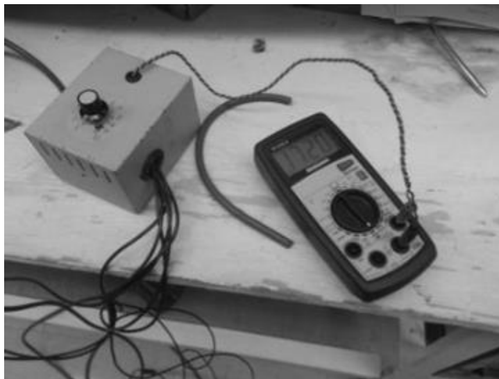
Figure 96: Switch and multimeter. The resistance of 1720 ohms represents room temperature
