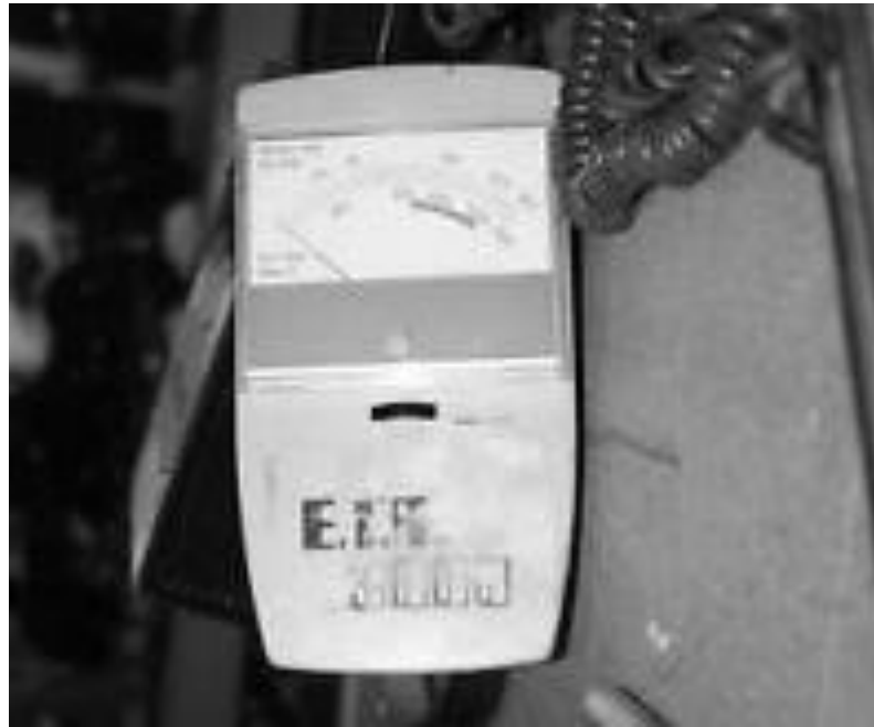
Figure 75: Airflow Industrial's E.T.A 3000 hot wire anemometer
