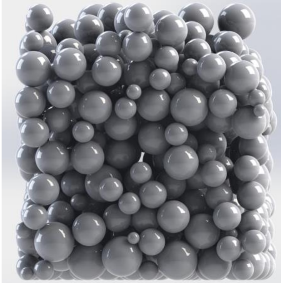
Figure 53: Full particle flow code model imported into the CAD/CAM environment before being processed for use as the verification model
