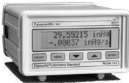
Figure 76: Paroscientific 746-16B pressure standard (Paroscientific, 2013)
