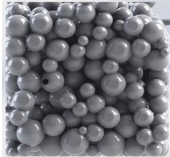
Figure 65: Rendering of the verification assemblage in the CAD/CAM software environment after constraints of printing size and thermal experiment preparation. Routes of insertion for one of the thermistors can be seen as a shadowed black circle. Width and height of the sample are both 7.62cm
