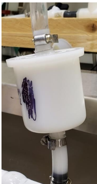
Figure 7-1: 5-micron filter showing a white slurry at input and a clear fluid at outlet
