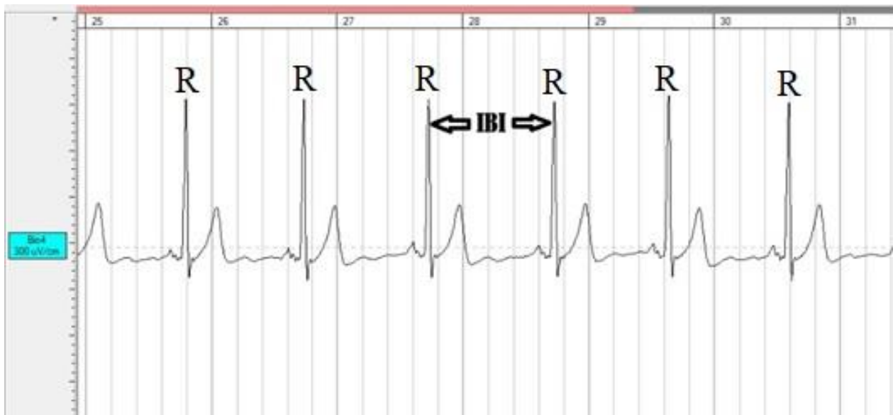
Figure 4. 1 Interbeat interval (IBI) and R-peak example in a raw ECG recording in WinEEG
