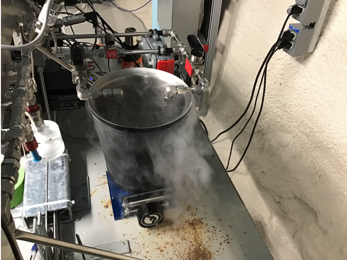
Figure 4.3: The Radon board with trap A submerged in liquid nitrogen.
