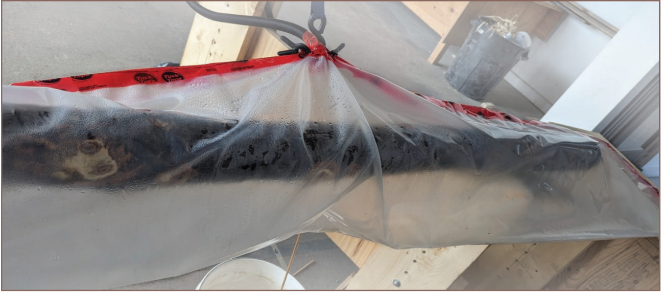
Figure 5.26 : Tree Steaming in Sealed Vapour Barrier Chamber
