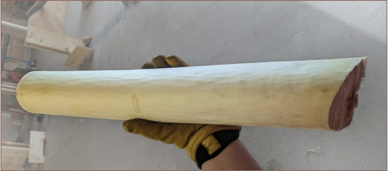
Figure 5.33 : Successful Steam Debarking Test
