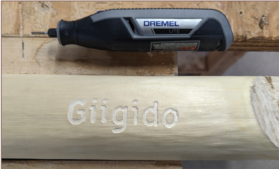
Figure 5.36 : Word Carving with Square Edge Dremel Bit When carving with a square edged Dremel bit, it is important to be conscious of the angle at which the bit touches the wood. This bit shape is unforgiving for angled contact and will yield uneven results if not handled with care. That being said, this bit allows a crisp and deep letter profile to be achieved easily.
