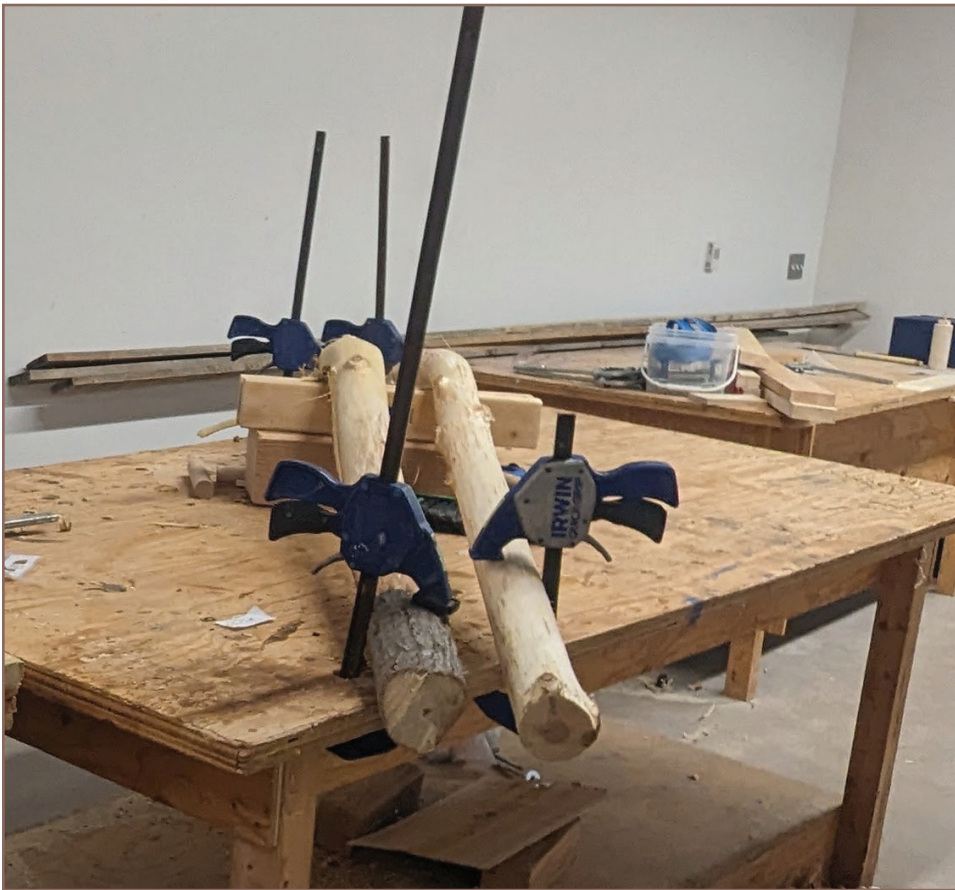
Figure 5.31 : Test Trees 1 and 2 Bent over Block Spacer
