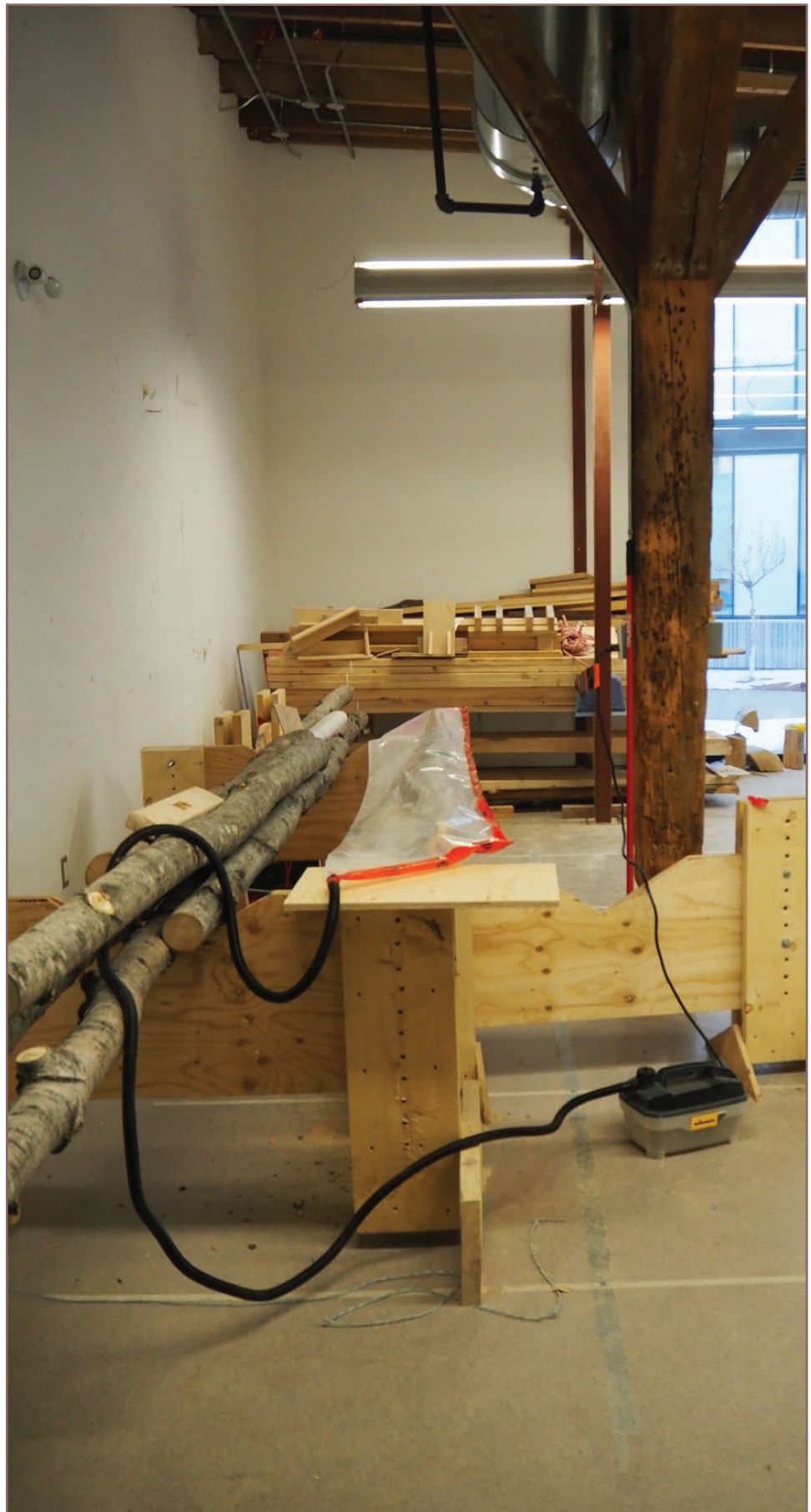
Figure 5.28 : Steamed Tree 1 Bent Over 8" Block Spacer
