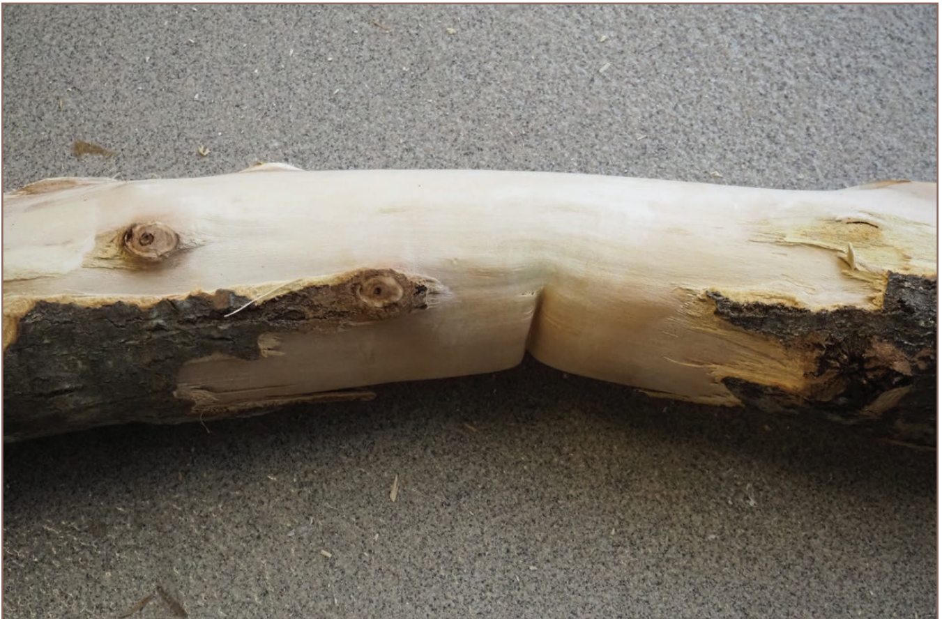
Figure 5.32 : Kinked Tree from Single Point Bending Technique
