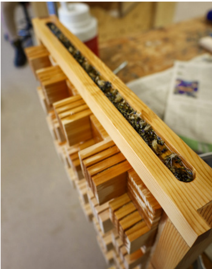
Routed trough with naughted twine, soaked in lavender buds and mineral oil mixture
