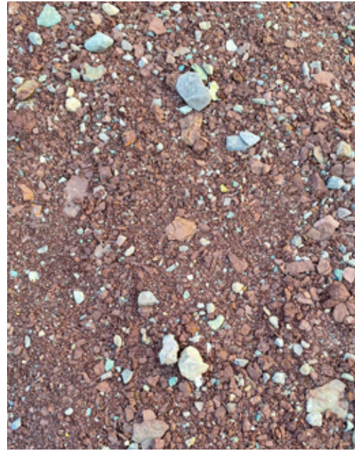
Figure 40: Red Shale found at the bottom of the drained Welland Canal in the winter months
