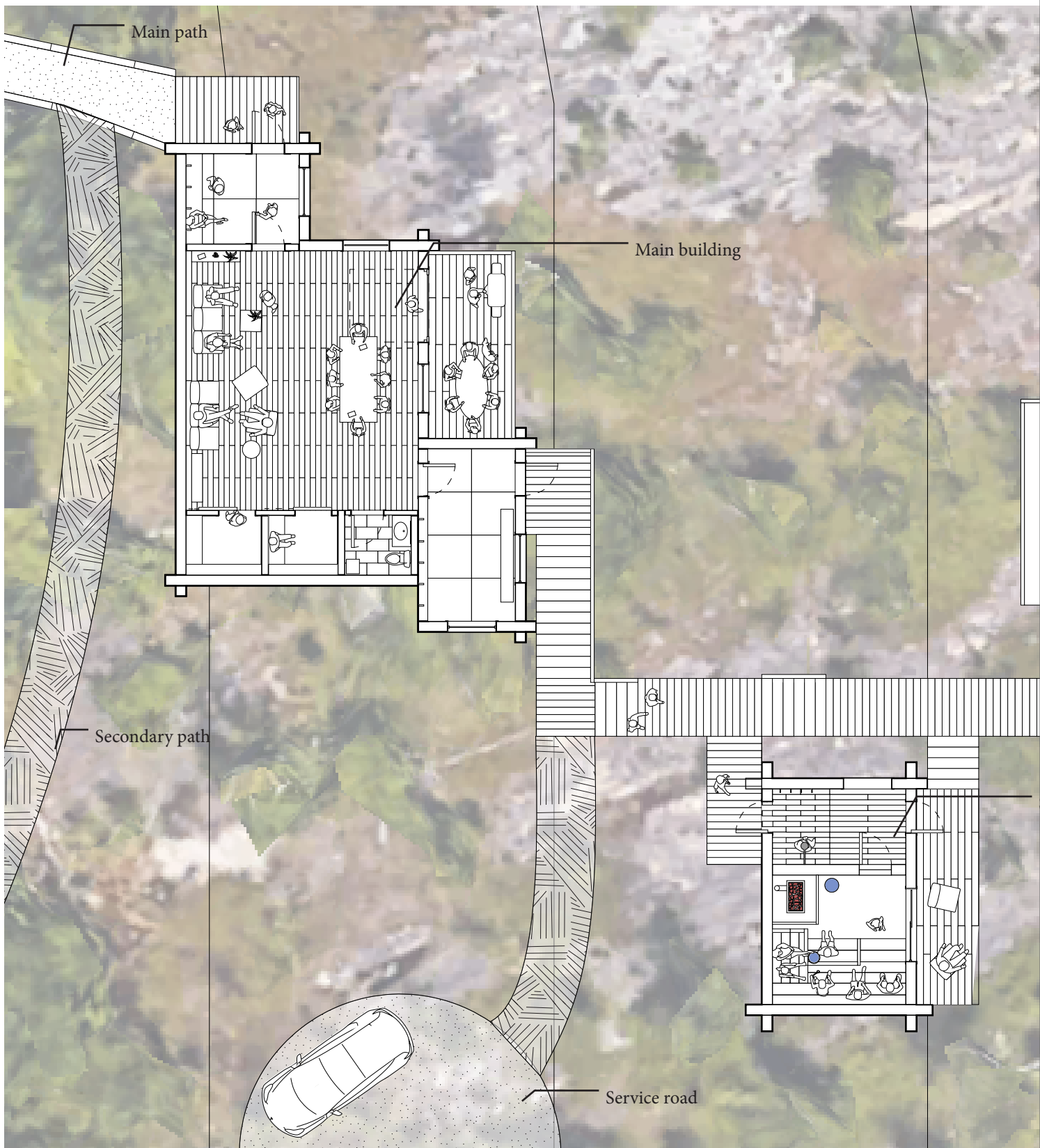
The floor plan shows the layout of the main building, sauna, community deck, dock with plunge into Ramsey Lake and the journey between each space. The service road allows for maintenance staff and users with limited mobility to have an easier access route to the main building and sauna. The pathway from the sauna to the dock is direct to allow users a fast and simple journey to cool down in the water.
