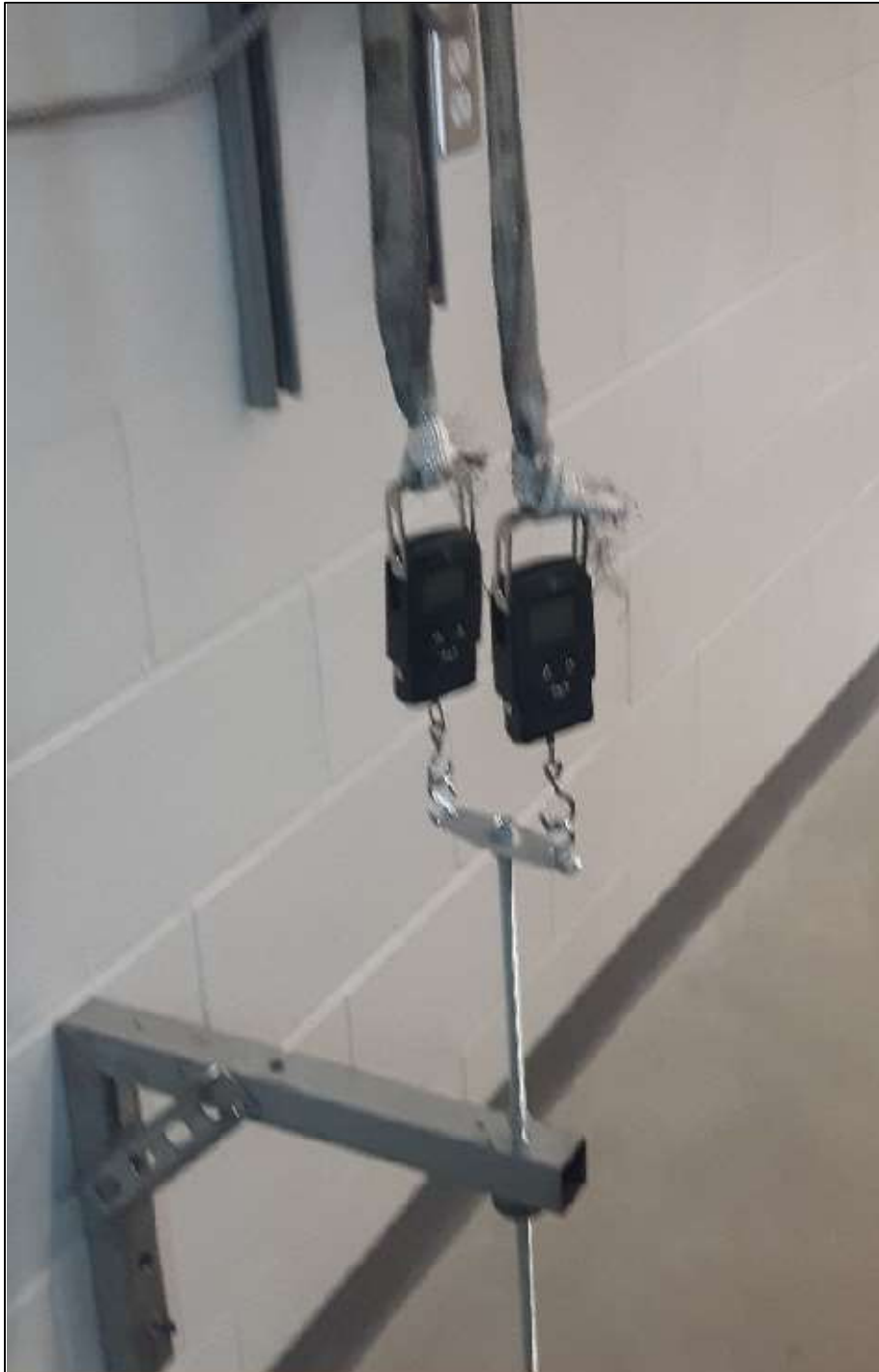
Figure 4.3: Dynamometer scales, attached to tension arm
