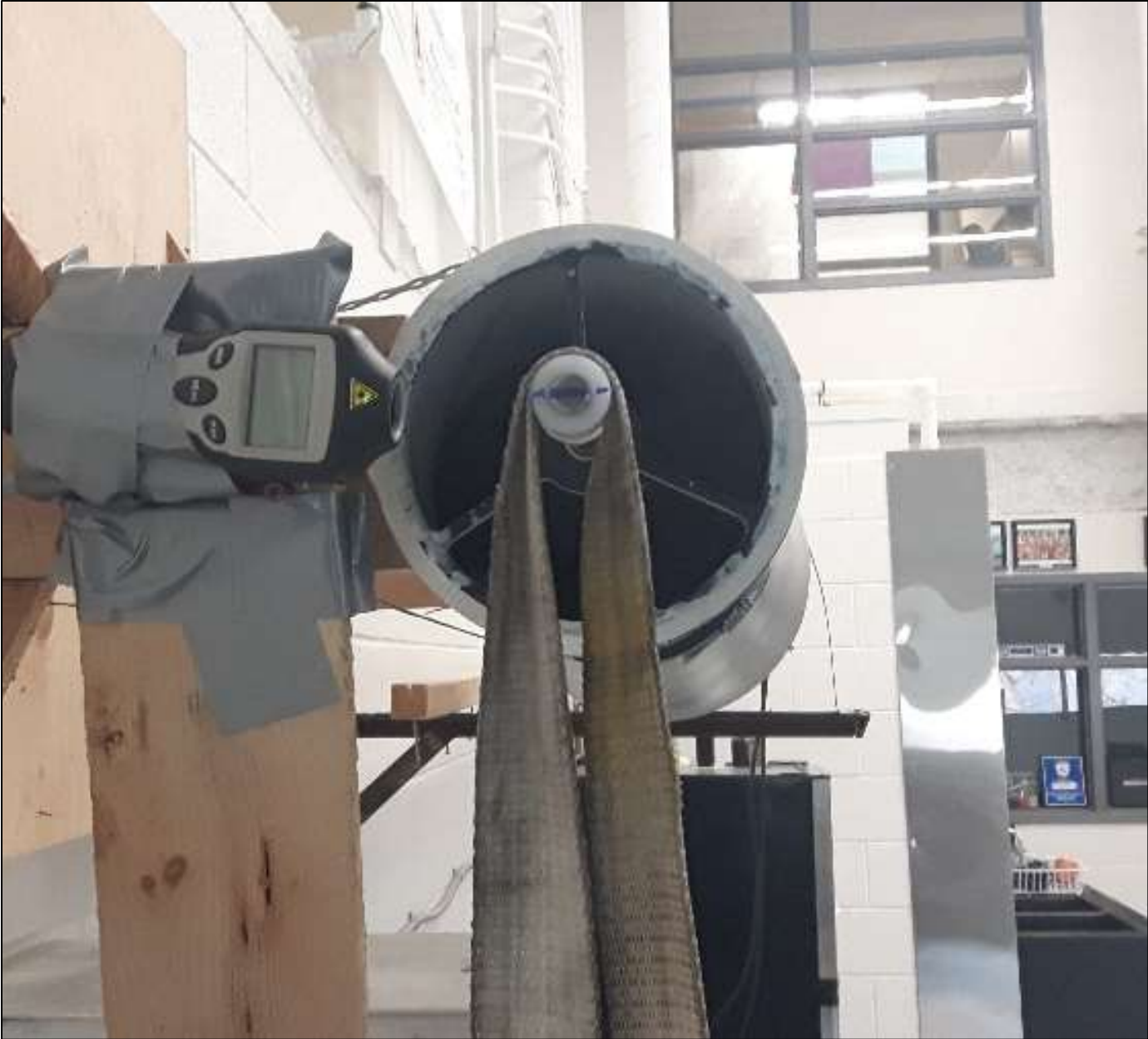
Figure 4.2: Dynamometer drum with cloth strap
