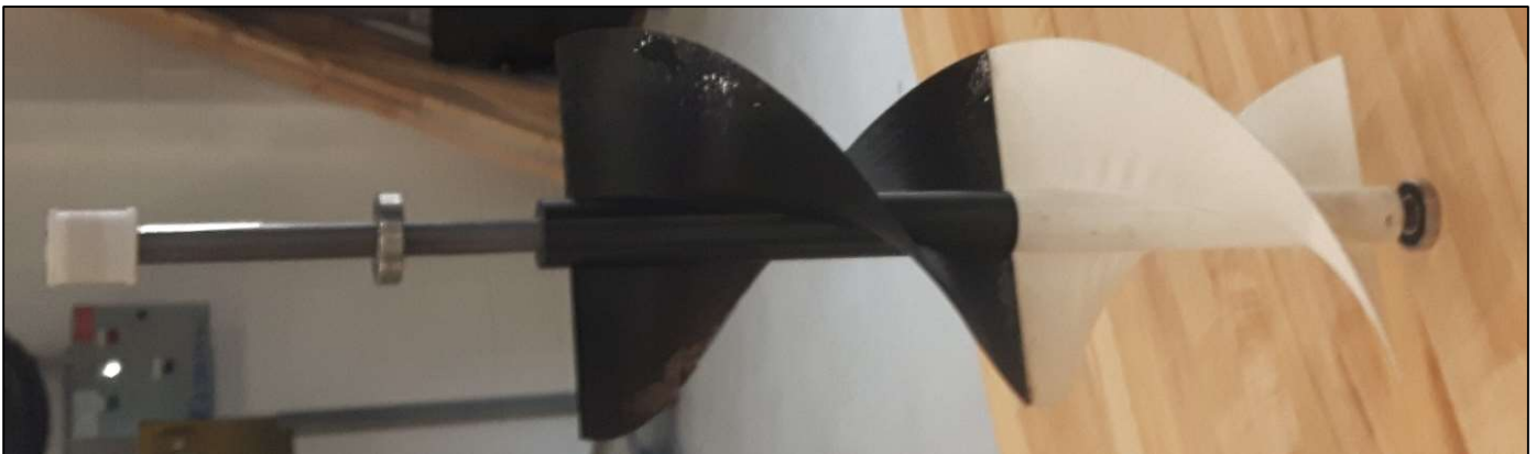
Figure 4.17: Blade, bearings and friction drum assembled on shaft
