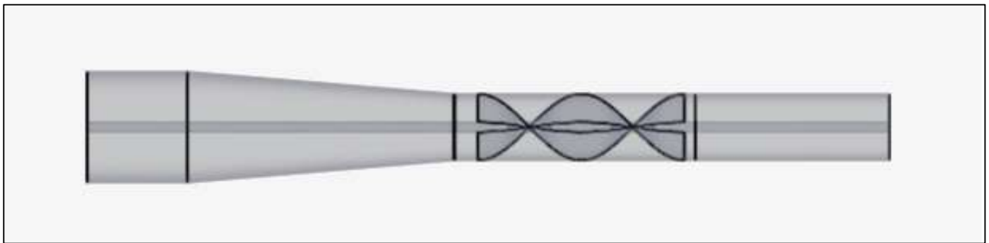
Figure 3.6: Geometry 2 (final test model); 4.56-degree half-angle diffuser
