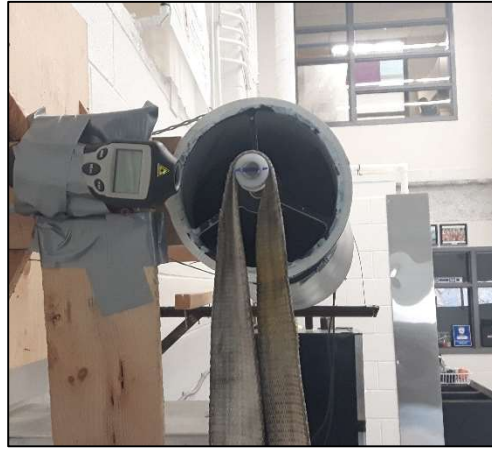
Figure E-1: Friction drum with tension strap (older tension strap used in calibration, photo is illustrative only)
