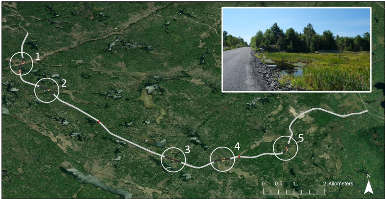
Figure 1.1: Aerial imagery of the study area includes the study road and surrounding wetland complexes along eastern Georgian Bay, Ontario. The 11.7 km study road is highlighted in grey, and the labelled white circles (1 – 5) identify Mitigated road sections. Each Mitigated road section consisted of ~ 300 m of paved road shoulders (dark grey sections) and ~ 100 m of rip-rap on road embankments (yellow sections) that are approximately centered within the 300 m paved section. Other wetland crossings that did not receive the mitigation strategy are indicated with red dots. The inset photo shows a Mitigated wetland crossing.
