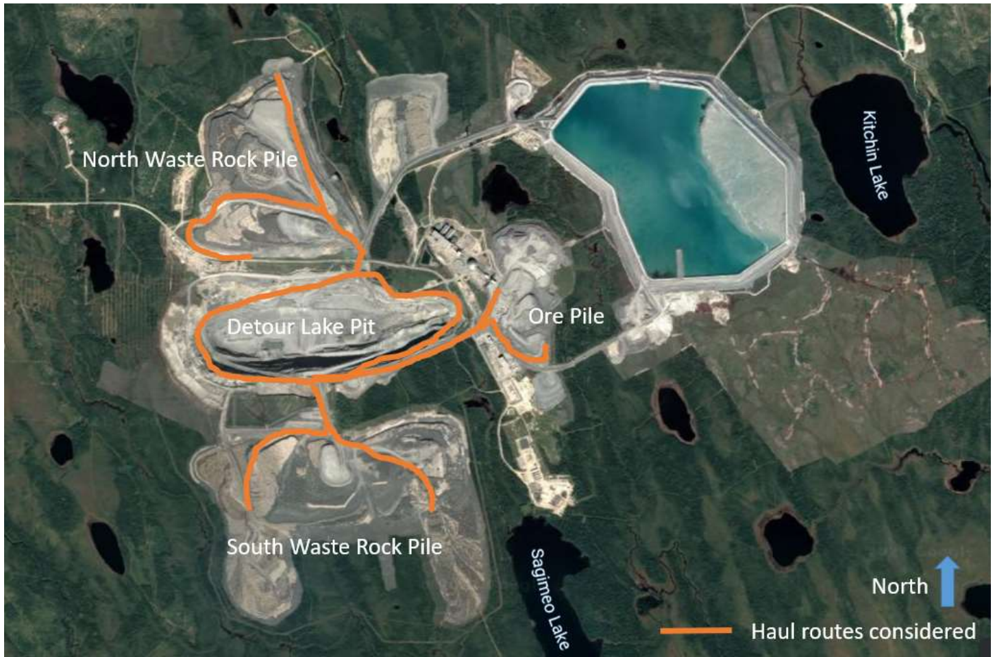
Figure 16. Main pit and dump point locations and assumed haul routes at the Detour Lake Mine site (Google Earth, 2021a).
