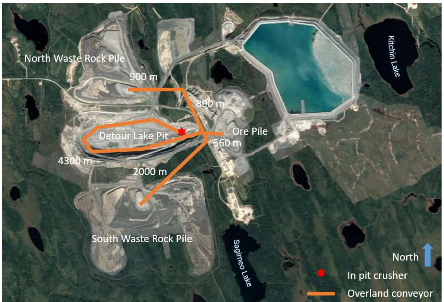
Figure 53. Location of in pit crusher and path of the overland conveyor along the main ramp to the various dump points.
