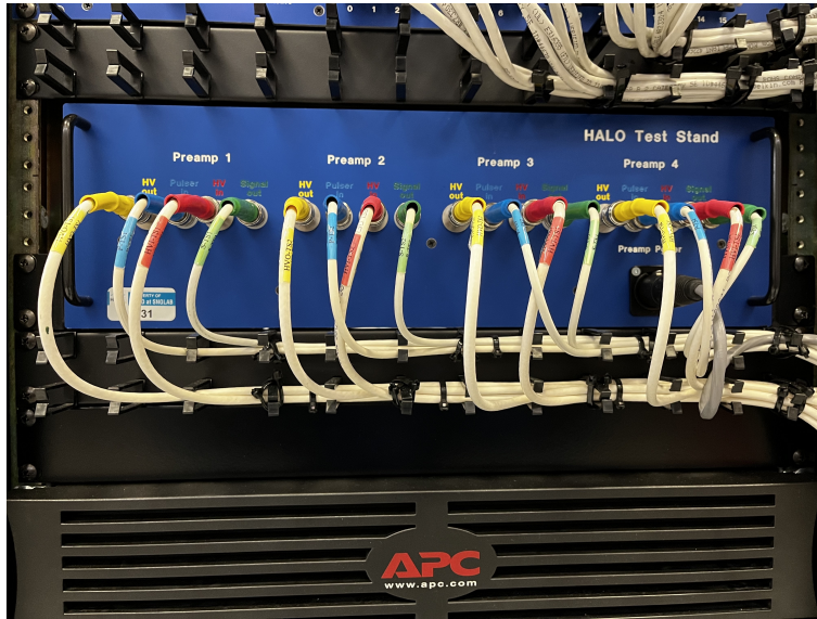
Figure 6.2: The preamp from the Test Stand to the DAQ system. Each chord is clearly labeled and colour coded.
