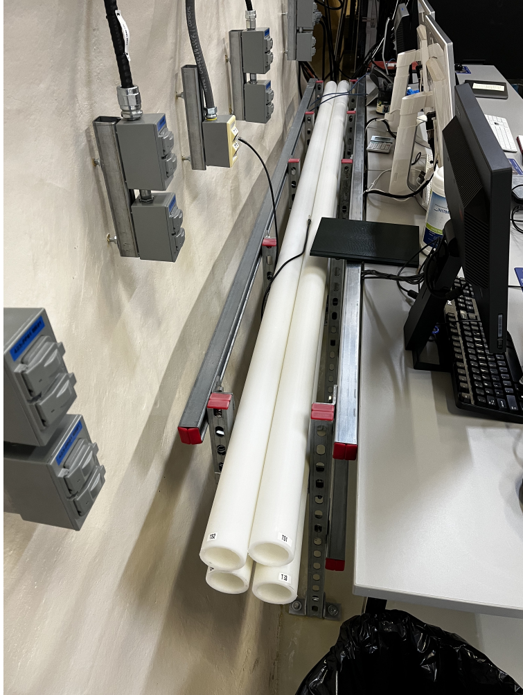
Figure 6.1: The underground test stand for HALO counters. The counters were placed in each of the four tubes. For the calibration run the calibration source was placed in the middle of the tubes.
