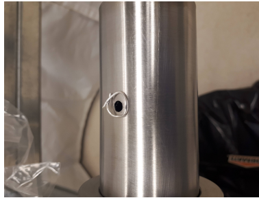
Figure 6.6: The counter after a hole has been drilled with the indium wire around the hole so the clamp will seal to the counter
