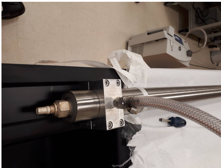
Figure 6.9: A prototype counter with clamp attached. It has a Tygon tube going in attached to a Helium leak detector that can be seen on the floor in the top right corner of the image.
