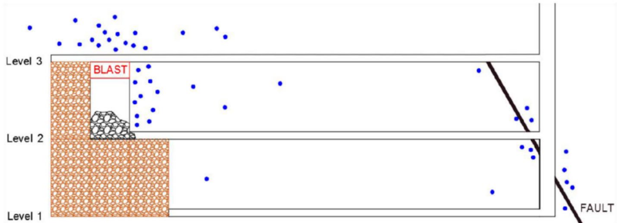
Figure 9 Seismic response of blasting illustrating induced events (blue) located near the blast and triggered events located on a fault distant from the mine blast (Brown, 2018)
