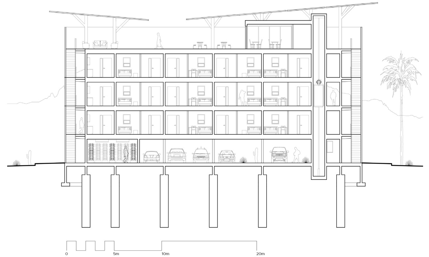
Fig. 112 Apartment section II
