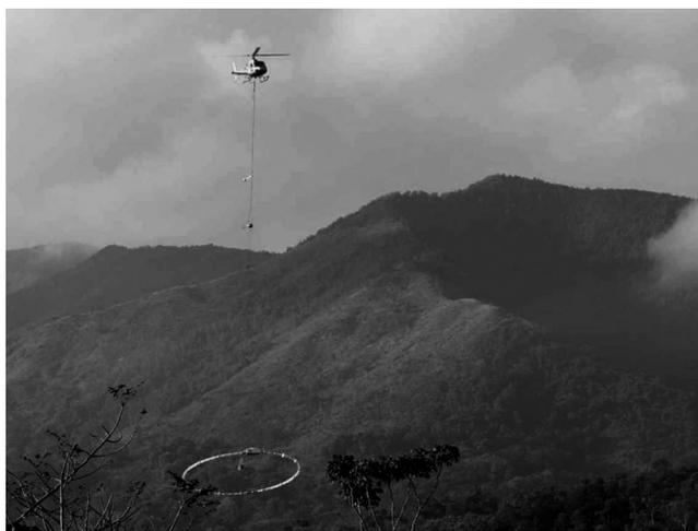
Figure 3. The HeliGEOTEM system acquiring data in the Dominican Republic. From Smith et al. (2009). Used by permission.
