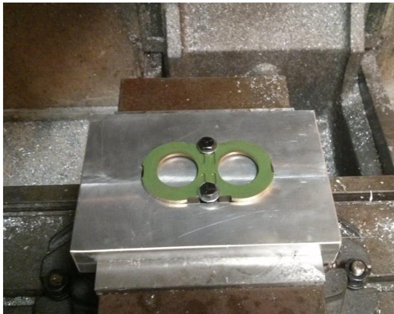
Figure 10: CNC Thrust Plate Machining Setup
