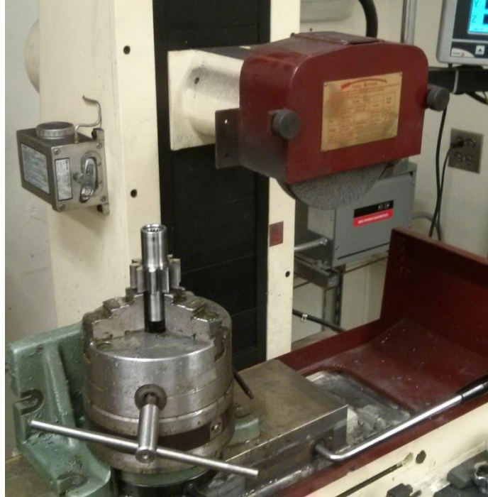
Figure 12: Surface Grinder Setup for Gear Wear Replication
