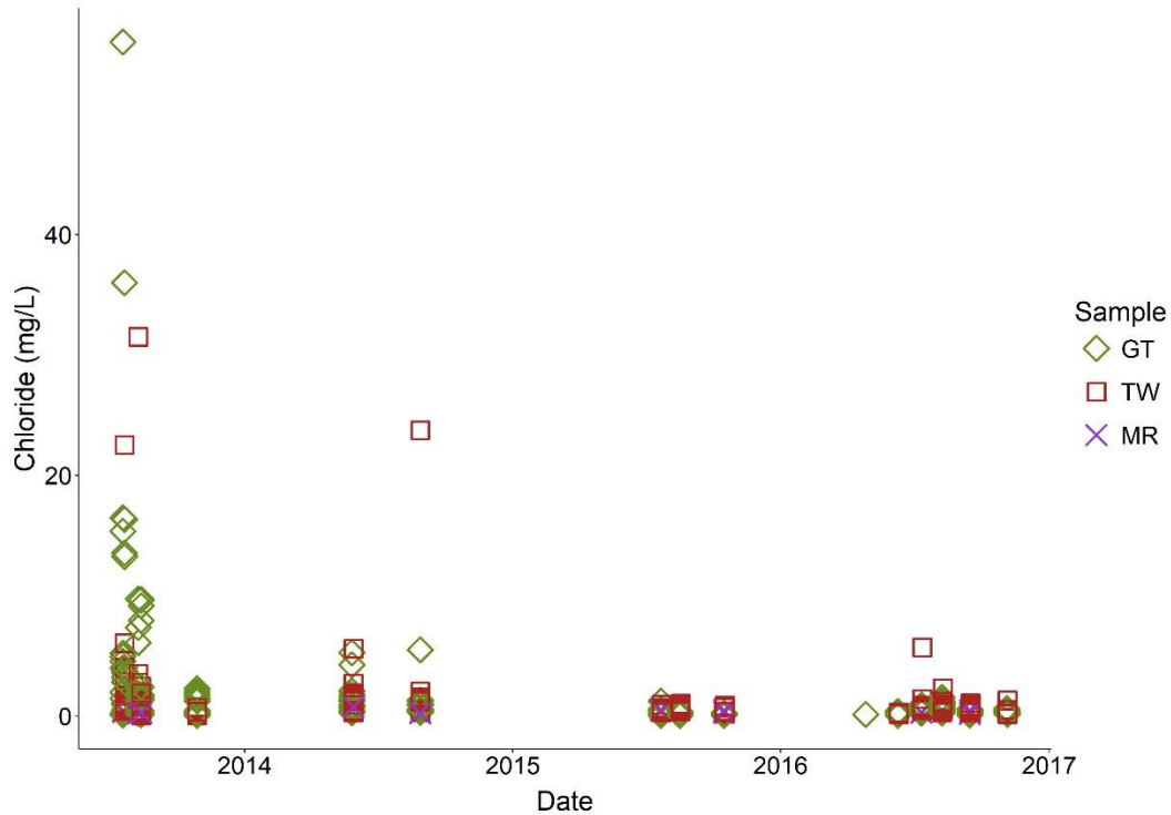
Figure A38. Concentrations of \text{Cl}^- (mg/L) from Technosol gravity through-flow (GT), Technosol tension water (TW), and Williams mine rock test cell (MR) water samples from July 2013 to Nov 2016. 12 samples < DL (0.03 mg/L).
