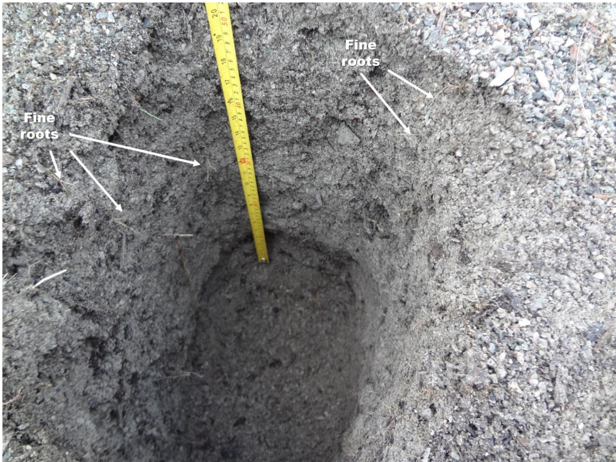
Figure 12. 40% organic, 60 cm deep, vegetated Technosol profile. Fine roots visible in upper layers of profile; little colour or structure variation seen with depth.
