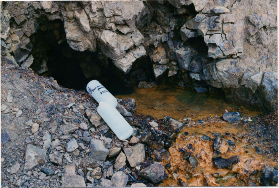
Plate 9: Precipitate formation in the Mike Horse creek bed before Station B9 without attached algae. October 23, 1989. (Around monitoring Station P4, Map 1)
