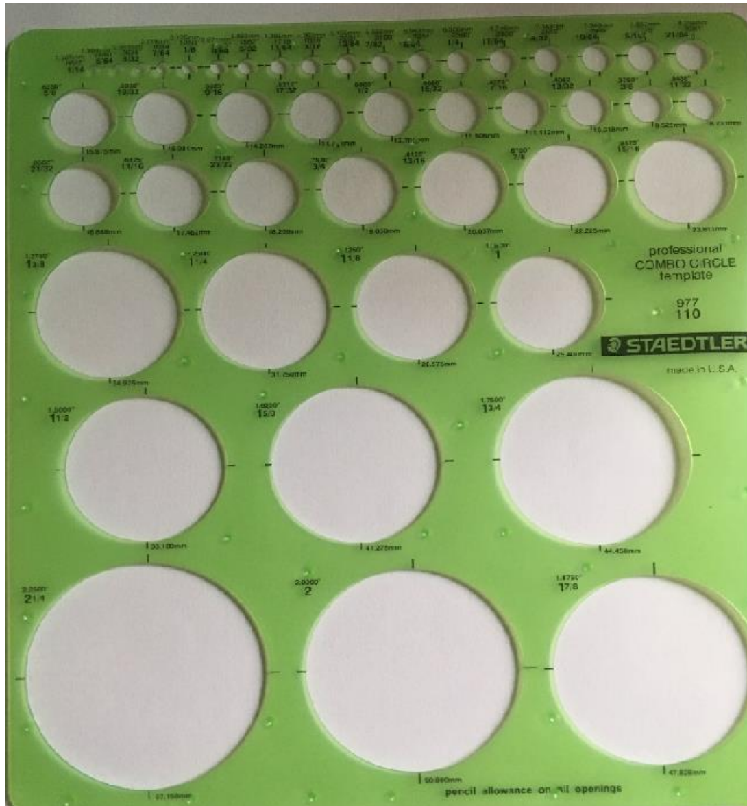
Figure 5: Circle stencil template. Illustrates Stencil template used in study, measured in millimeters.
