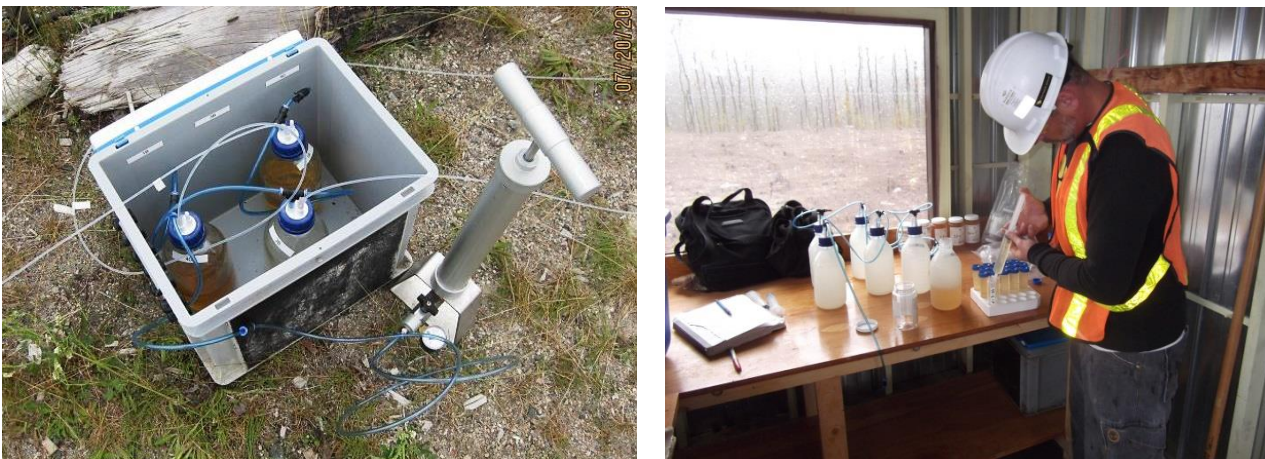
Figure 32. (L) Suction plate lysimeter systems were pressurized with a hand pump to collect water samples contained within the Technosol. (R) Water samples collected via tension plate lysimeters being prepared for transportation to ELFRS for analysis.
