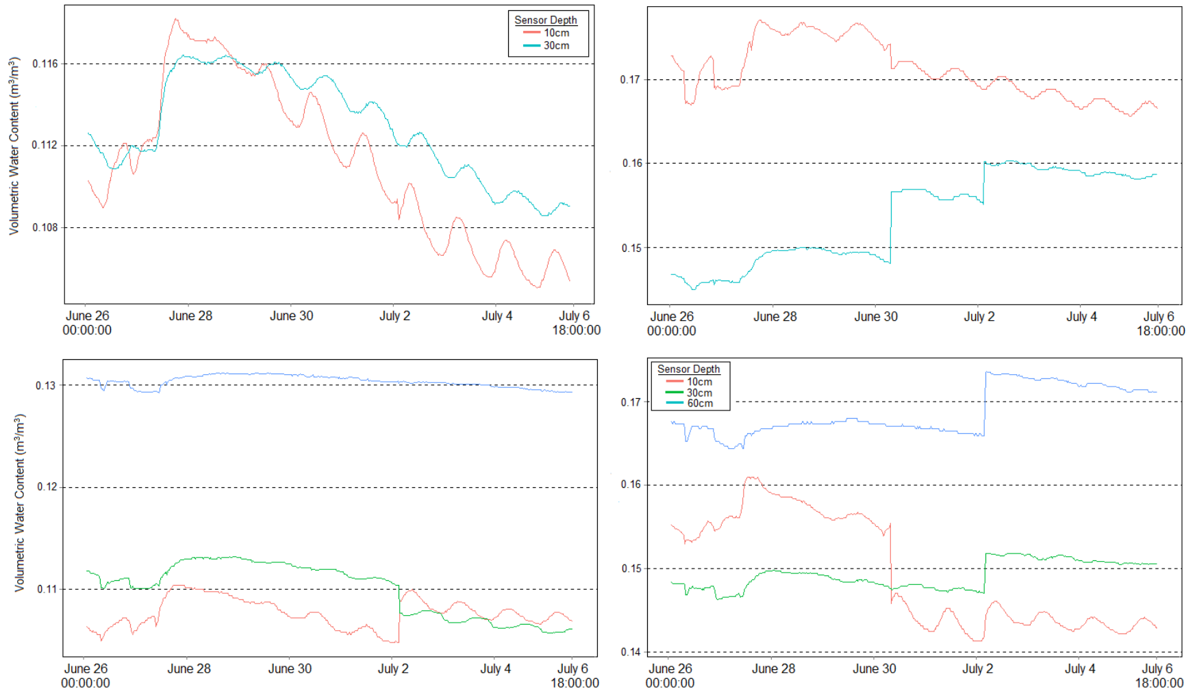
Figure 45. Soil moisture changes in two Technosols of 30 and 60 cm depths, after a low intensity, long duration precipitation event on June 26, 2013. Plots are ordered from 1 (top left), Plot 2 (top right), Plot 3 (bottom left) and Plot 4 (bottom right). n = 3 for each sensor depth.
