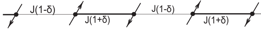
Figure 1.2: The dimerized spin chain. The arrows represent the spin at each lattice site, and thick and thin lines represent the modulated exchange couplings J(1 + \delta) and J(1 - \delta) , respectively.
