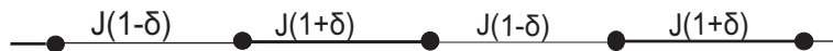
Figure 4.1: A spin chain with an alternation of strong and weak bonds adapted from [14].
