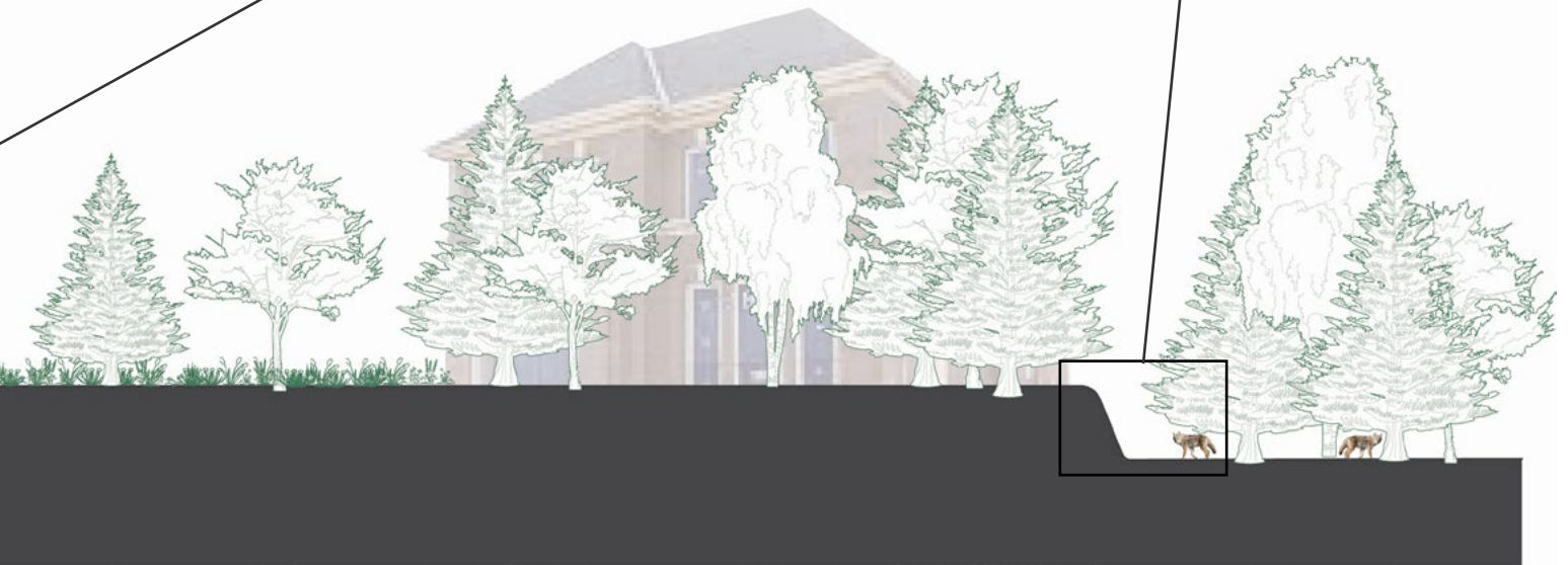
Figure 53: Berm Design - Coyote Barrier.
