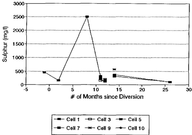
FIGURE 4.15b: Historical variation in sulfur concentrations sampled from different test cells.
