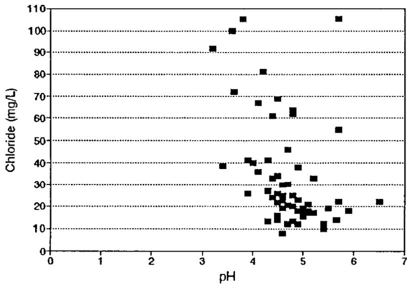
FIGURE 3.2: pH vs. chloride at station 2016.
