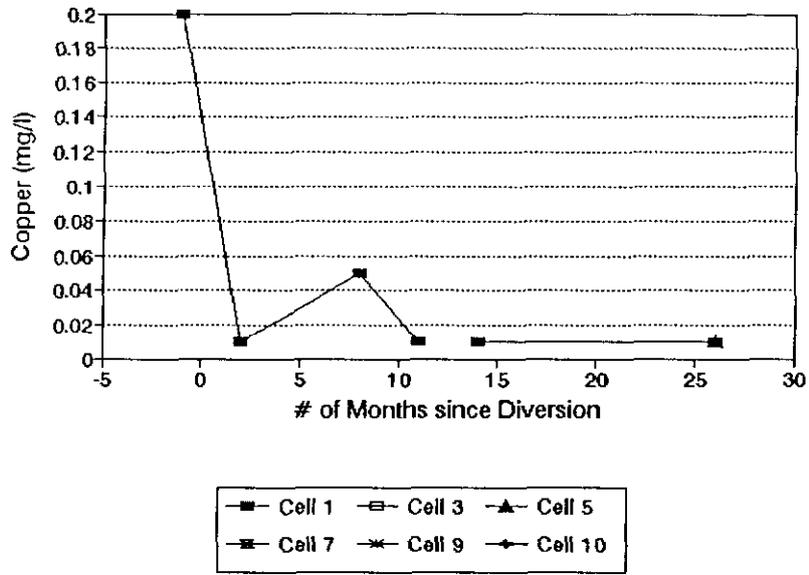
FIGURE 4.16c: Historical variation in copper concentrations sampled from different test cells.
