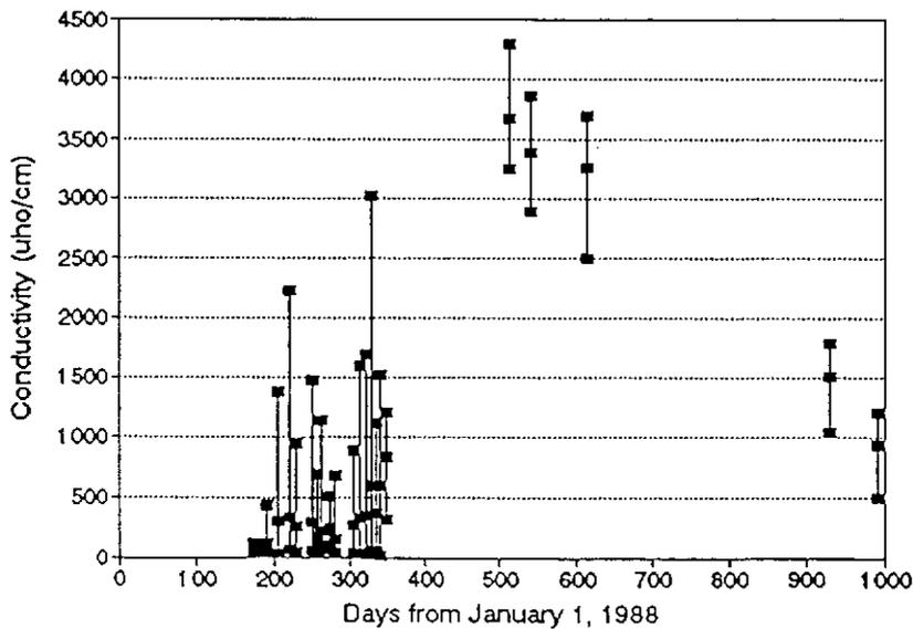
FIGURE 4: B) Water conductivities in the bog. Each vertical line indicates the minimum, mean and maximum conductivity measured from all stations in the water quality sector on a given date.
