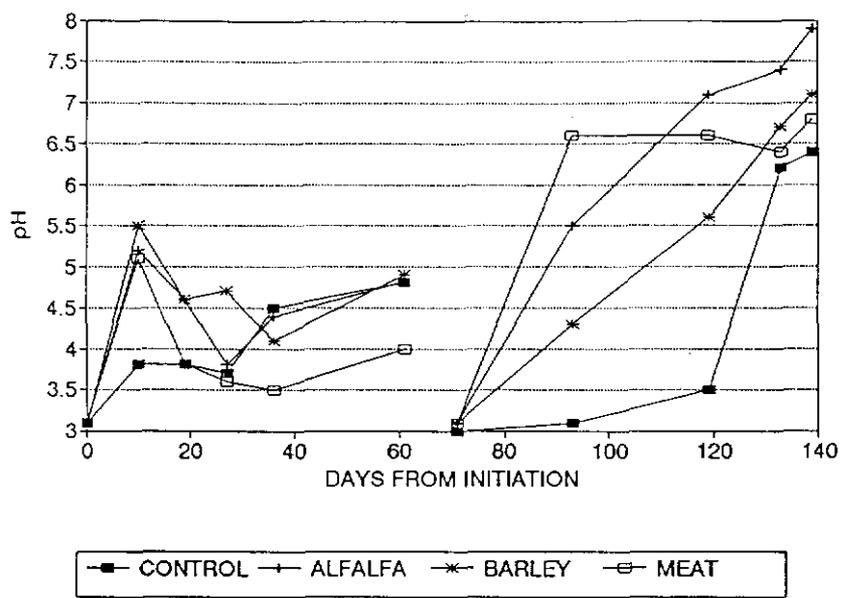
FIGURE 6: Change in pH with time in 15 mL vials. Vials contained AMD/bog water and a variety of carbon amendments. Water in the vials was replaced on day 60 and the vials restarted on day 70.
