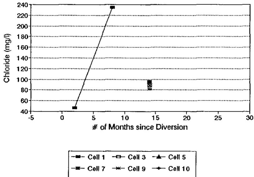
FIGURE 4.15c: Historical variation in chloride concentrations sampled from different test cells.
