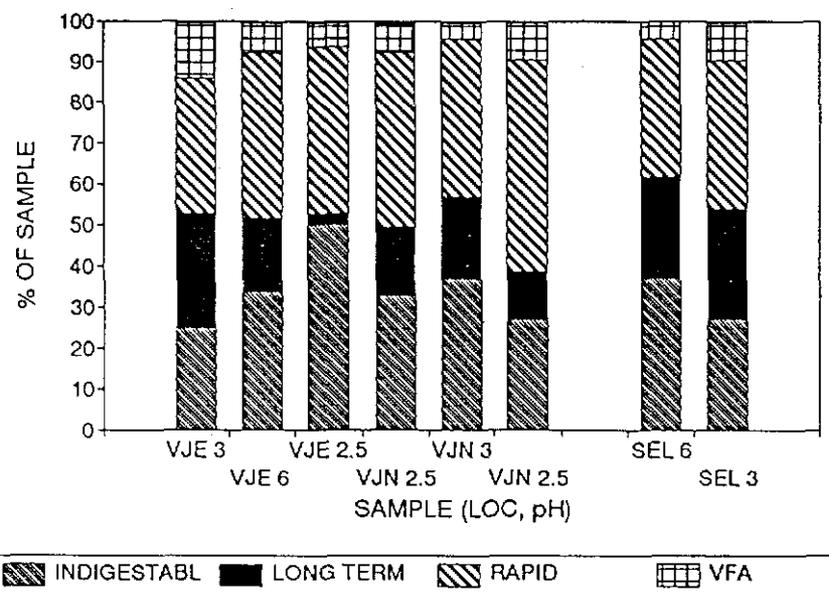
FIGURE 7: Percentage of an amendment sample which is extractable by acetone (VFA), hydrochloric acid (RAPID), and sulphuric acid (LONG TERM). That which is left over is assumed to be INDIGESTIBLE.
