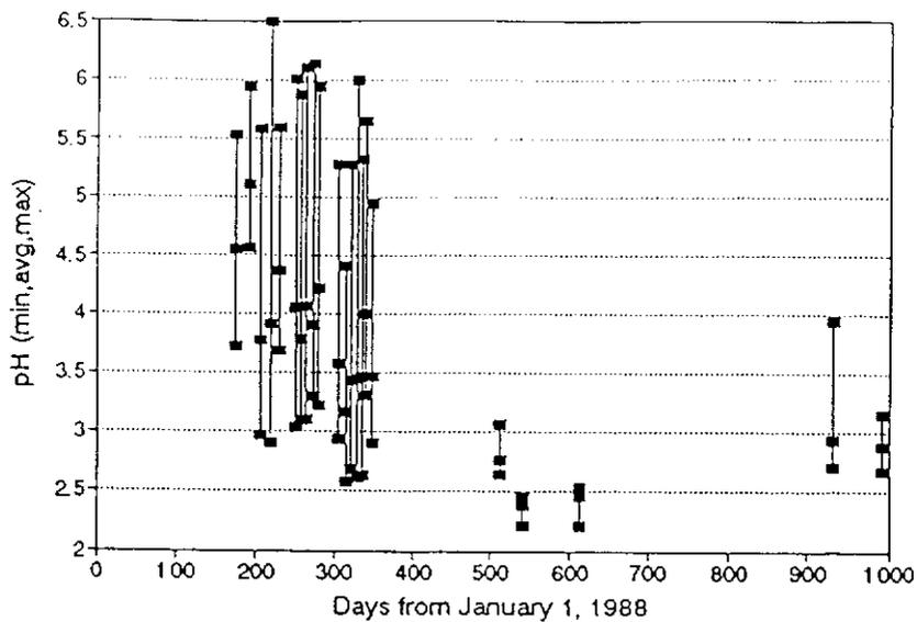
FIGURE 4: A) Water pHs in the bog, compiled from the water quality sector. Each vertical line indicates the minimum, maximum and logarithmic mean of all stations in the water quality sector on a given date.
