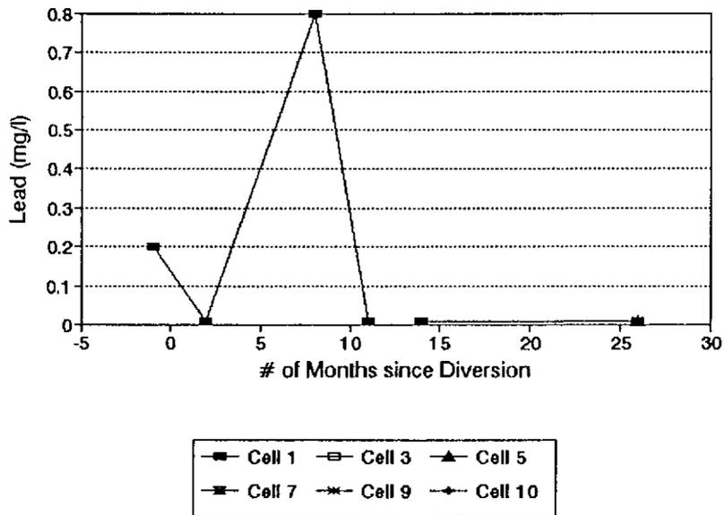
FIGURE 4.16b: Historical variation in lead concentrations sampled from different test cells.
