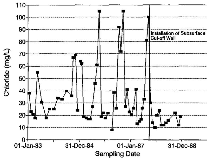
FIGURE 3.6d: Historical chloride concentrations at station 2016, from 1983 to 1990. Note significant summer drop since 1988.
