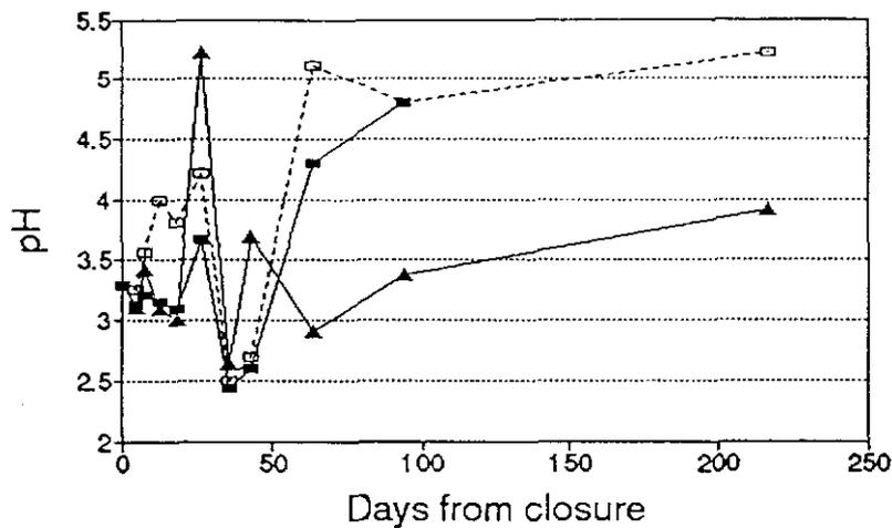
FIGURE 5: Change in pH with time in 4.2 L jars. Jars contained carbon amendment and AMD/bog water. Jar water pHs measured at given dates after closure. Old A (solid squares) and Old B (open squares) indicate that amendment received old amendment water before closure. New (solid triangles) indicates that the jar received fresh AMD/bog water at the time of closure.
