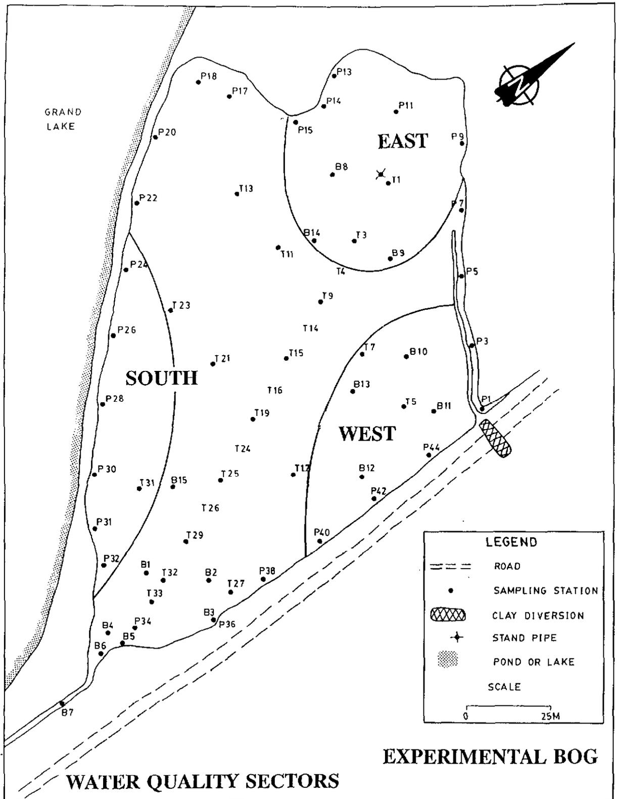
MAP 4.1: Overview of the Experimental Bog showing permanent water monitoring stations and statistical sectors.
