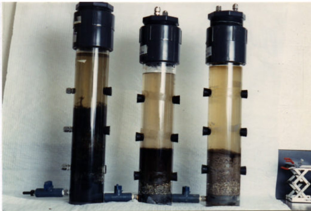
Plate 2: 1993 Laboratory reactors used to study biological arsenic removal
